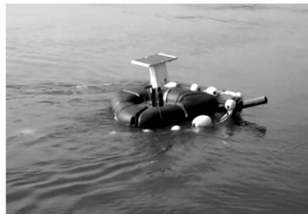
(b) 流速为 1.2 m/s 的姿态 the reef status in current of 1.2 m/s
