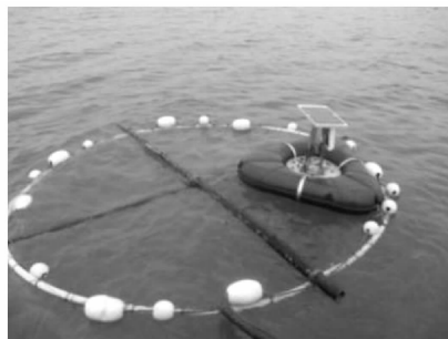
(a) 静水中姿态 the reef status in stillwater
